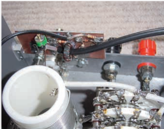
Fig. 7: The s.w.r. sensing p.c.b. is mounted on the back of the input socket.
