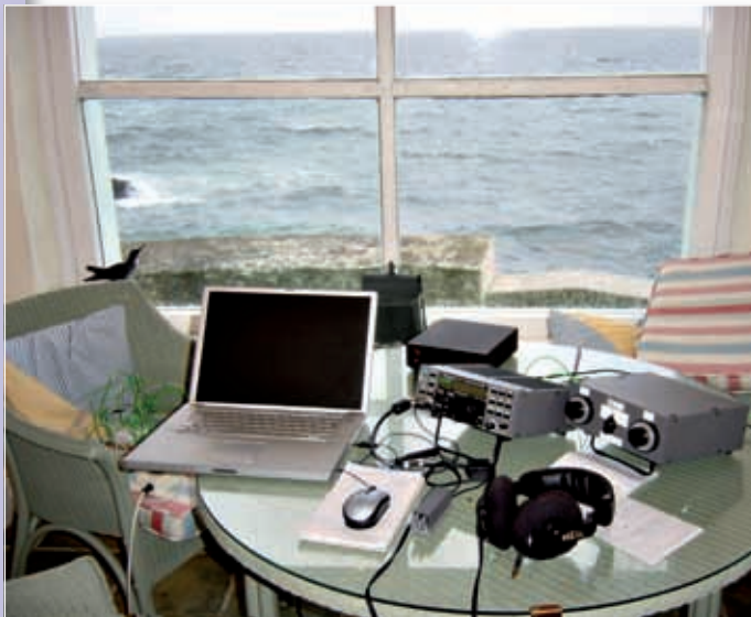
Operating position at St Anthony's Point, Cornwall in May 2006, when a 61m doublet was tuned by the balanced EZ-match tuner (right), in its K2/100-matching box.
